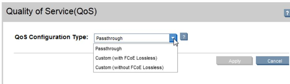
Note: You cannot switch to Custom (without FCoE Lossless) when the domain has a fabric associated with an FCoE capable interconnect module, a Shared Uplink Set has an associated FCoE network, or a server profile has an FCoE connection.
