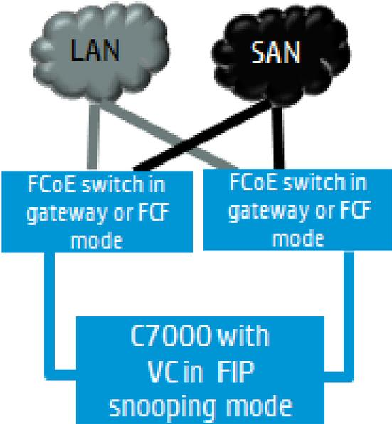
Virtual Connect SUS configuration when using FCoE
