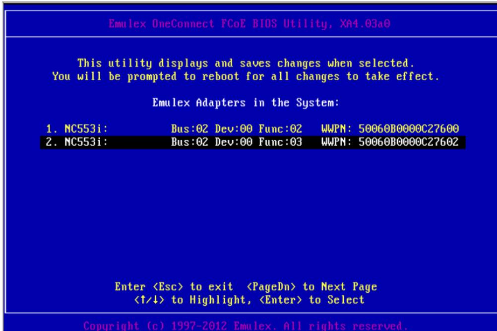
16. Use the arrow keys to choose the second adapter and repeat the previous steps to view the WWPN of its target controller.
