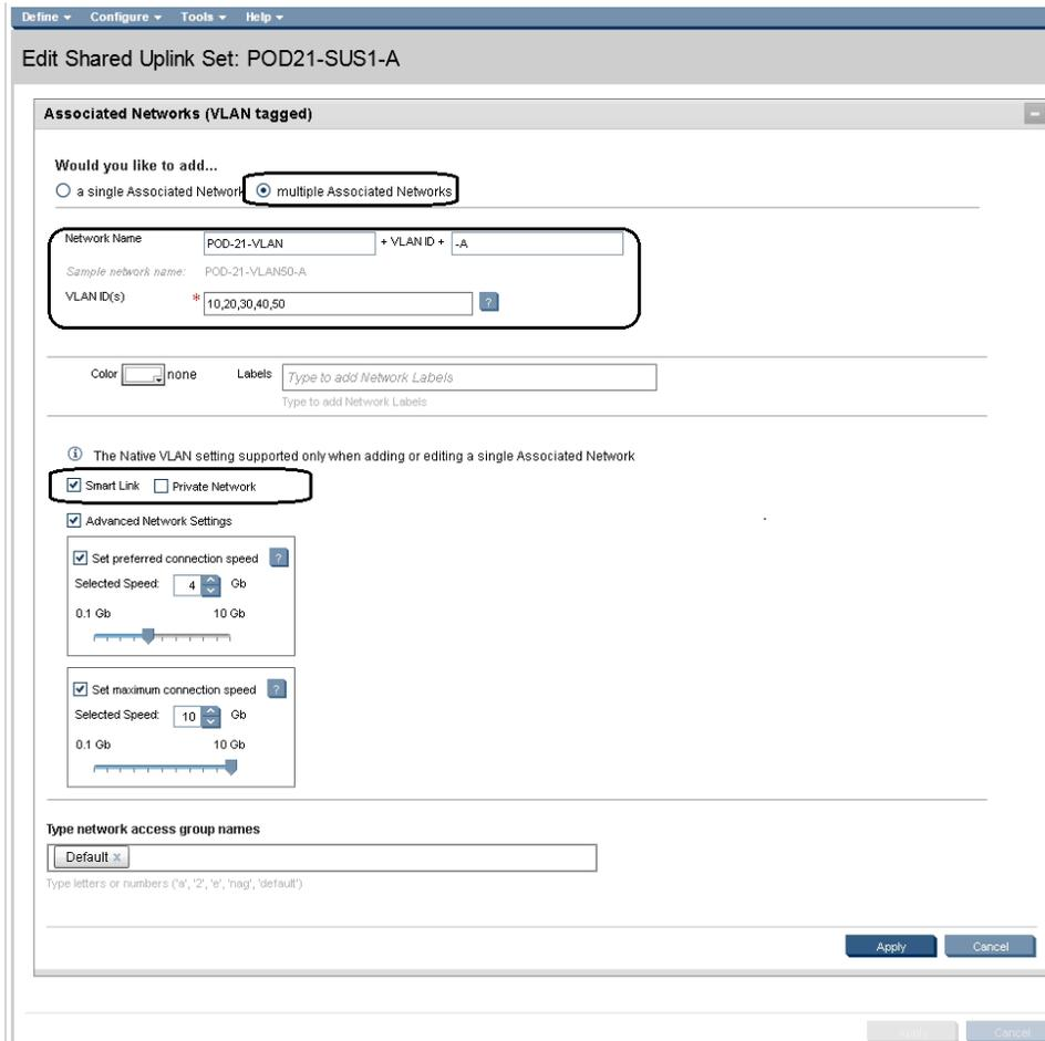
11. After you complete the data entry, the Associated Networks section of the window should display as follows.
