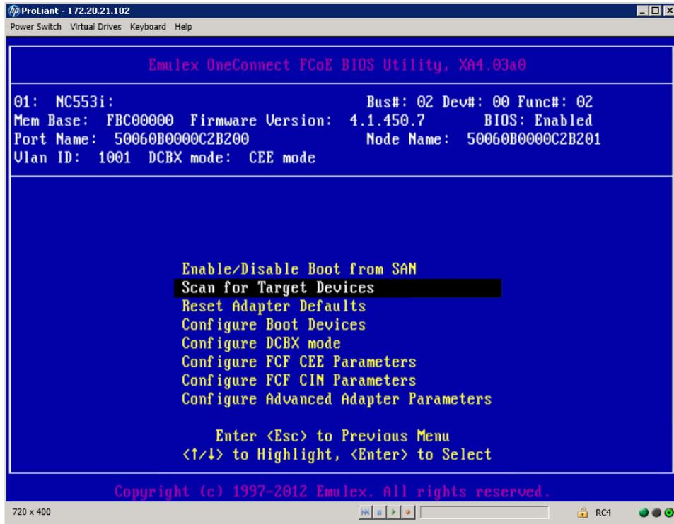
13. Arrow down to Configure Boot Devices and press <Enter> to view its configuration.
