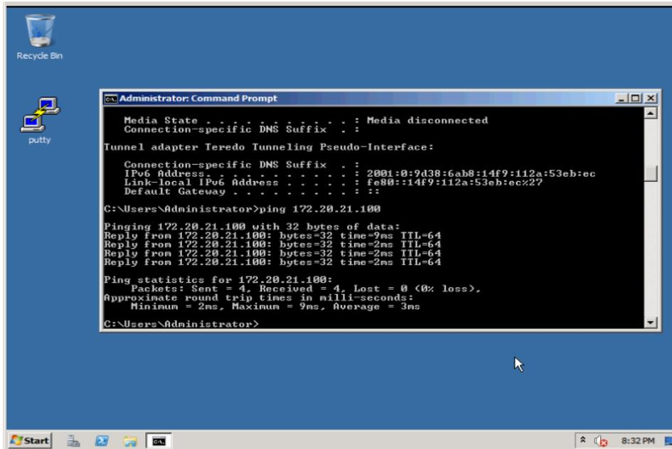
7. Optionally, if you wish to test Virtual Connect Uplink fail-over and the effect it has on the server, you could start a ping -t 172.20.xx.100 in a command window, then Edit the vNet and drop the "Active" uplink and save the network.
