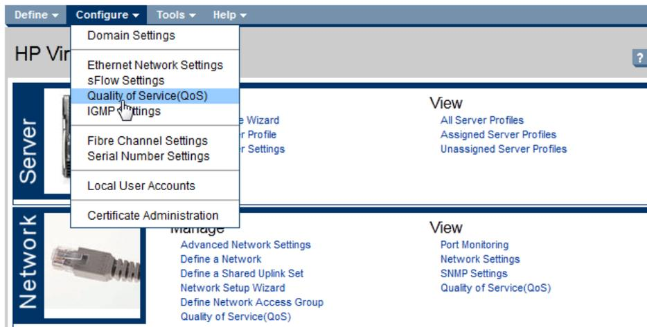
Under the QoS section you select the QoS configuration type. This specifies the QoS operation mode. The default mode is “Pass-through”. If FCoE is not being used, select Custom (without FCoE Lossless), by doing so, you free up an extra queue that would normally be assigned to Lossless FCoE. However; if FCoE connections have been created or will be used, then select Custom (with FCoE Lossless). For this lab, select Custom (with FCoE Lossless)
