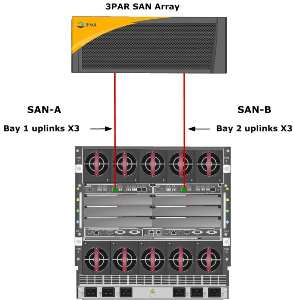
Physical view of the Fibre Channel connections without SAN Fabric
