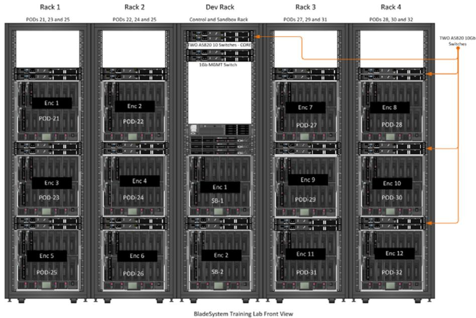
Each POD is configured with a c7000 Blade enclosure, TWO FlexFabric modules and TWO 5820 10Gb LAN switches configured in an IRF cluster. An EVA SAN is connected through FlexFabric ports X1 and X2 to a Brocade SAN fabric and a 3PAR storage array is directly connected to the FlexFabric Modules, port X3, for "FLAT SAN" connectivity.
