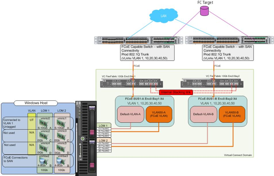
In this lab, both port trunks are active because they are assigned to separate SUSs. Although it is not done in this lab, additional uplinks could be used to increase uplink bandwidth and provide additional availability.
