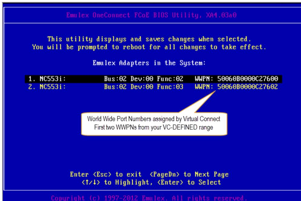
12. Highlight the top adapter using the keyboard arrow keys and press <Enter> to view its configuration.
