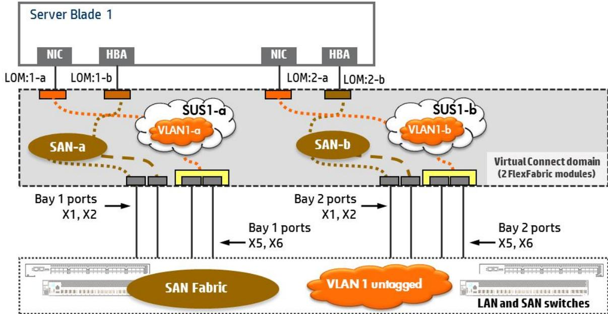
**Figure 2: Logical View of the Virtual Connect Networks and SAN Fabric Configurations**
