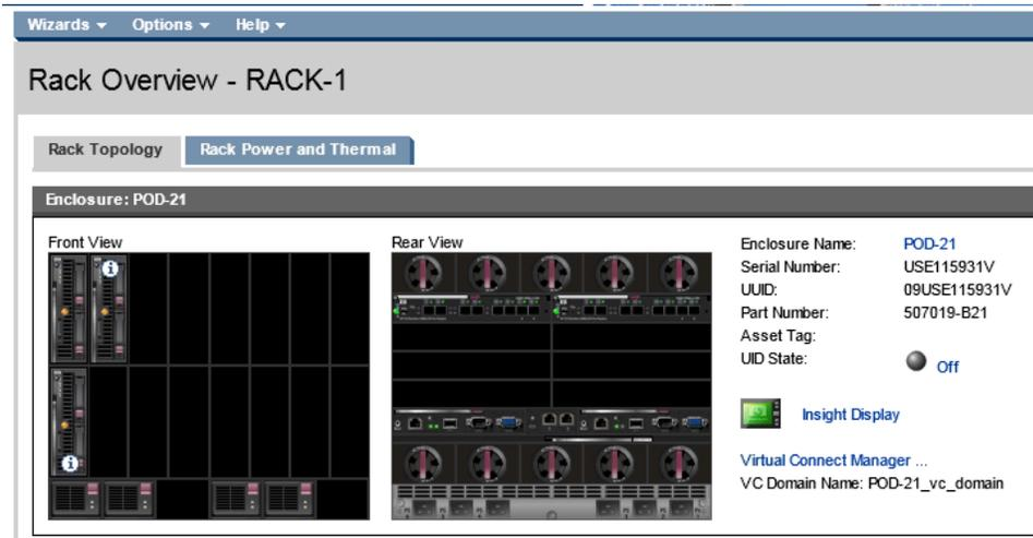
3. Click on the server in Bay and select the Virtual devices tab and press "Momentary Press". As the server is booting, Select "Integrated Remote Console" from below and open an iLO Session with the server.
