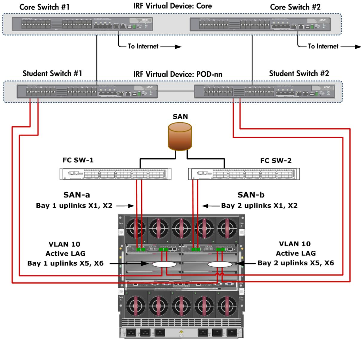
Figure 1: Physical view of the Fibre Channel connections
