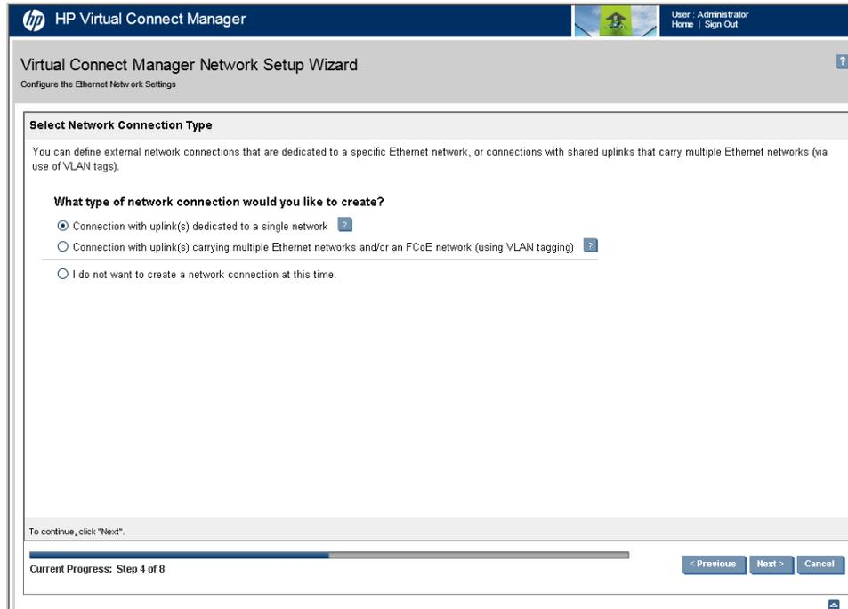
17. In the define a single network screen create a network called Network-1. Do not enable SmartLink or VLAN Tunneling, add Uplink X4 from Bays 1 and 2 modules and Click Create Network. Then **Click Create Network** on the following screen.
