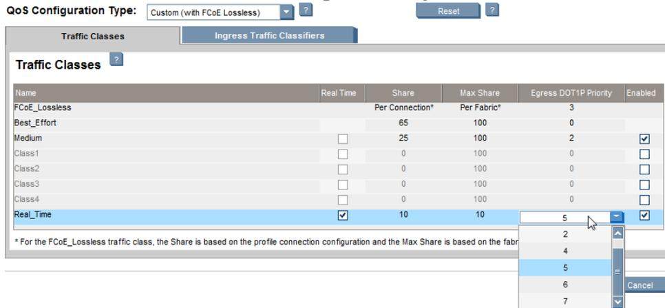
**Note:** Please make sure that if you use FCoE on uplinks, the FCoE traffic from the upstream device is already marked with an 802.1p value of 3 when it reaches the VC module as you cannot change this setting in Virtual Connect.
