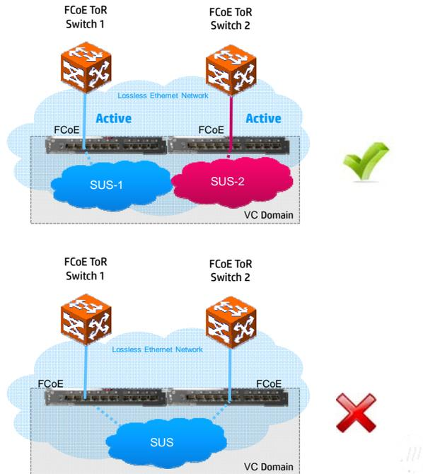
**Note:** FCoE-capable Shared Uplink Sets must always contain ports from a single VC module in order to maintain the SAN-A/B isolation.
