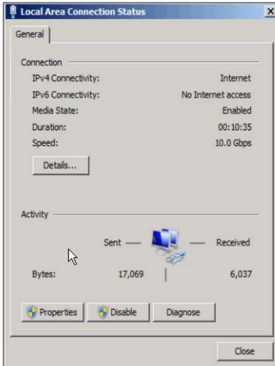
Notice that the Speed field corresponds to the Virtual Connect maximum speed for the FlexNIC, not the minimum.
