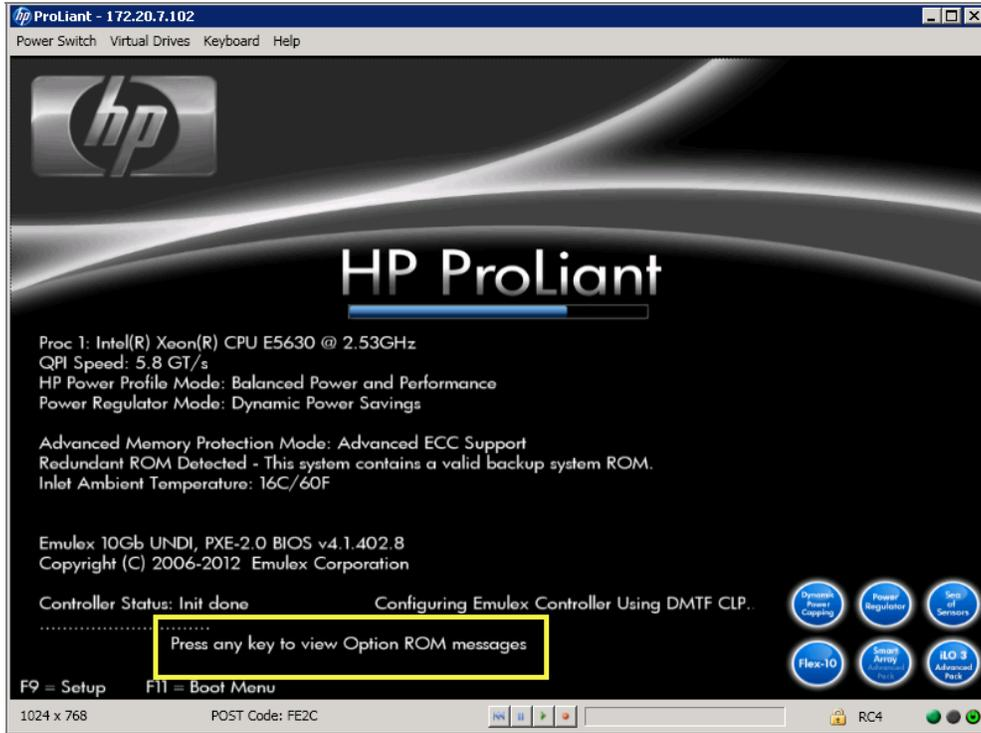
To verify the Emulex BIOS configuration was modified by the Server Profile you examine the settings applied to the adapters by Virtual Connect. During the POST processing stage, you will see a prompt to “Press any key to see POST Messages.”
