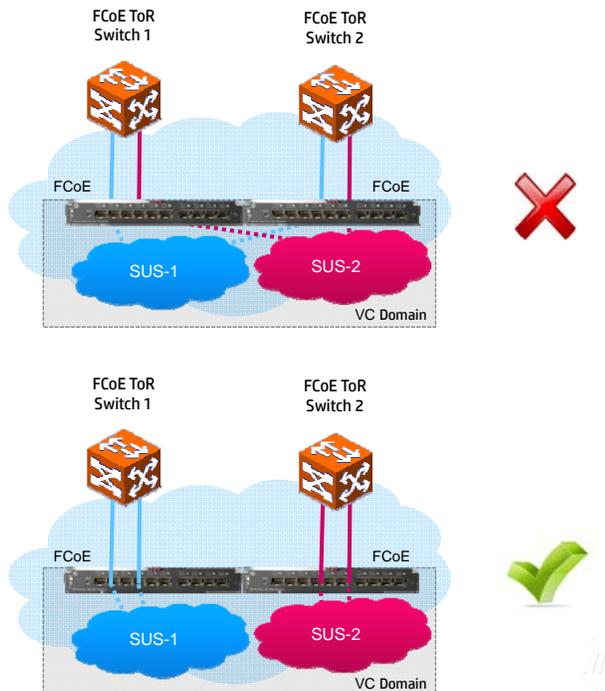
**Note:** FCoE-capable Shared Uplink Sets must always be connected to a single Top of Rack switch in order to maintain the SAN-A/B isolation.
